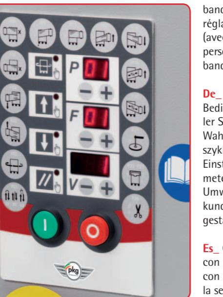
**En** Microprocessor control panel with digital display to select wrapping cycle and adjust machines parameter (possibly change and save the wrapping cycle).
